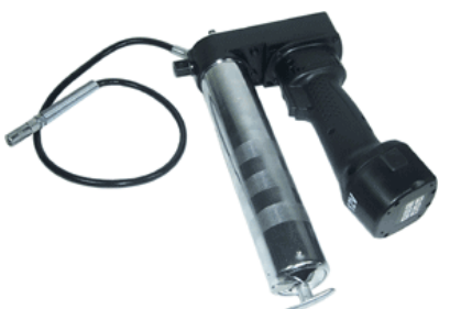
A2000 12V Cordless Grease Gun, 500cc bulk fill or 400g cartridge. Max 6000 psi.
